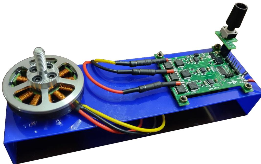
Figure 1 Y-CYC-ESC demo kit hardware
